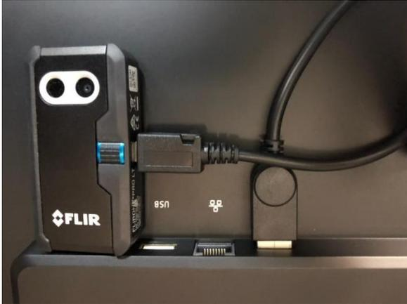
Use the USB to female MicroUSB adapter and connect the FLIR Thermal using the male port to the XDS-2285.
