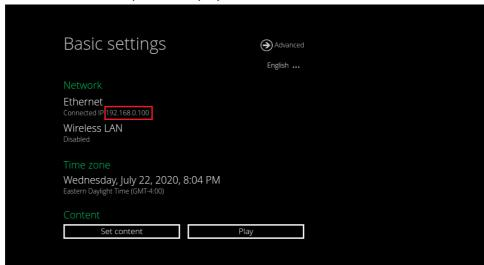
To get connected to the Sensor (Which IP is 192.168.0.250), make sure the IP of the panel is using the same network ID 192.168.0.XXX. Change the IP setting on your Router or contact your network administrator if you don't have the same network ID.
