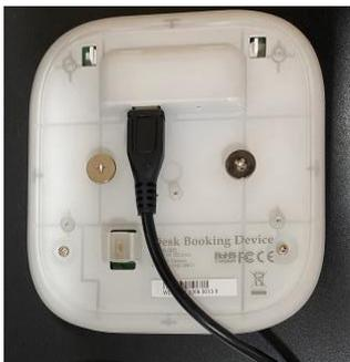
3. Install the **back cover** and use the **Cable Route Slot** for cable management:
