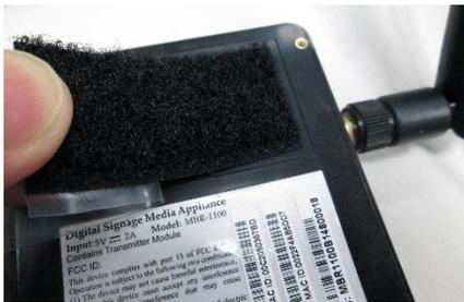
2. Stick the other Velcro pad onto the back of monitor, and then attach the player to it. Use HDMI extension cord to connect player and the monitor.
