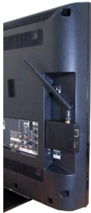
**Mounting Option 3: [Attach the player on the back of the monitor using Velcro]**
