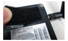
2. Stick the other Velcro pad onto the back of monitor, and then attach the player to it. Use HDMI extension cord to connect player and the monitor.
