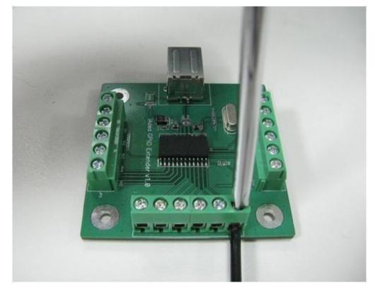
3. Fasten the terminal block with screw driver:
