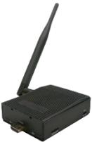
**Attach** the wireless antenna as shown in left, screw antenna clockwise onto the post
